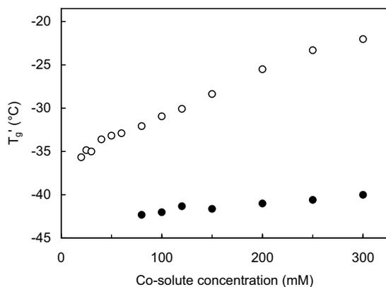
Fig. 2. Effects of sodium tetraborate (○) and boric acid (●) on  $T'_g$  (glass transition temperatures of maximally freeze-concentrated solutes) of frozen mannitol (50 mg/ml) solutions ( $n = 2$ ).
