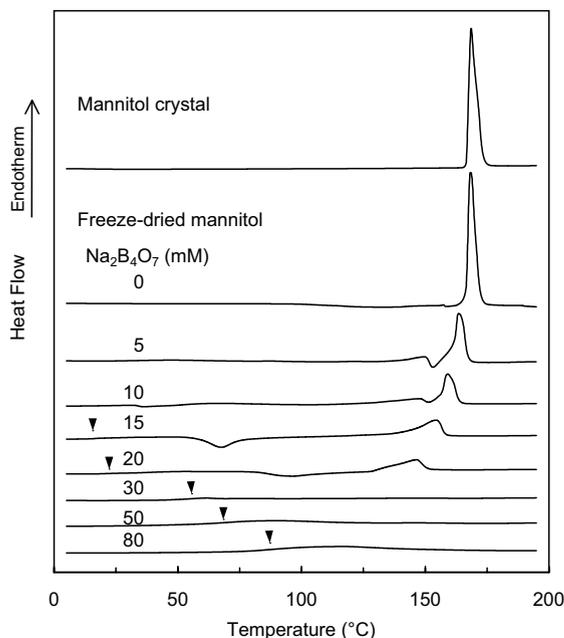
Fig. 4. Thermal profiles of freeze-dried mannitol (50 mg/ml) and various concentration sodium tetraborate combinations. Freeze-dried solid (0.8–1.4 mg) in an aluminum cell was scanned at 10 °C/min. Glass transition temperatures are marked with inverted triangles (▼).
