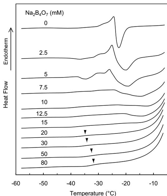
Fig. 1. DSC scans of frozen aqueous solutions containing mannitol (50 mg/ml) and different concentrations of sodium tetraborate. Glass transitions of maximally freeze-concentrated solutes ( $T'_g$  values) are marked with inverted triangles (▼).
