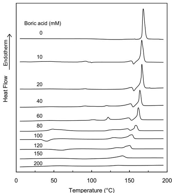
Fig. 6. Thermal profiles of freeze-dried mannitol (50 mg/ml) and various concentrations of boric acid combinations. Freeze-dried solid (0.8–1.4 mg) or mannitol crystal (1.03 mg) in an aluminum cell was scanned at 10 °C/min.
