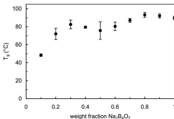
Fig. 5. Glass transition temperatures of co-lyophilized mannitol and sodium tetraborate combinations (25 mg/ml total) as a function of composition. Freeze-dried solids (0.5–1.0 mg/ml) were scanned from –20 °C at 10 °C/min. Symbols represent measured midpoint values  $\pm$ S.D. ( $n = 3$ ).
