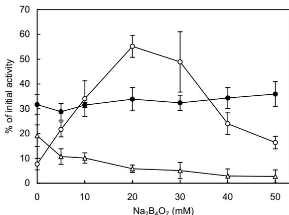
Fig. 8. Effects of excipients on the relative activity of freeze-dried LDH. Aliquots (10  $\mu$ l) of LDH (0.01 mg/ml) solutions containing 10 mM sodium phosphate buffer (pH 7.0) and various co-solutes were freeze-dried. Each symbol and error bar represent the mean  $\pm$  S.D. ( $n = 5$ , ( $\Delta$ ) w/o polyol, ( $\circ$ ) 50 mg/ml mannitol, ( $\bullet$ ) 50 mg/ml sucrose).
